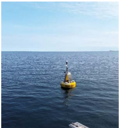
Buoy recording wave, current, lake temperature, and weather conditions offshore of Station Beach.
